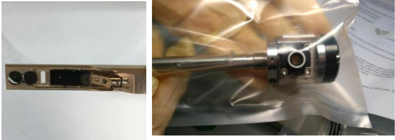
Fig 2 The actual MEMS aperture holder for Sorter phase element
